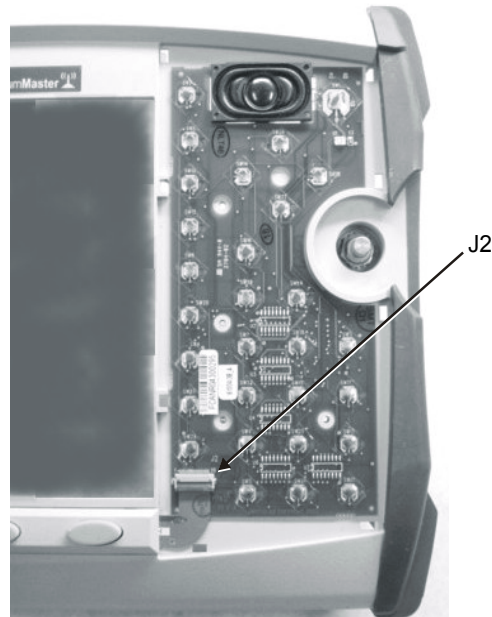
Figure 3-10. Main Numeric Keypad Connector J2
