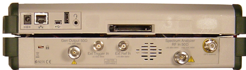
Figure 3-6. MS272xB Case Halves Partially Separated
